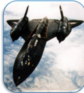
**The Ultimate Physical Limit (1976):** Proved to be heat from air friction, sufficient to soften airframes' aluminum alloys at high speed. The SR-71 Blackbird spy plane (right) reached 2,193.2 mph (the official record). Some of its surfaces reached 800°F, necessitating titanium alloy construction and the use of special fuel as a coolant – in spite of operating in the cold, thin air above 80,000 feet.
